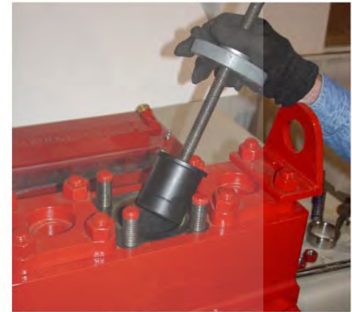
6.) Insert the tri-pin puller head, all pins retracted, into the discharge seat.
