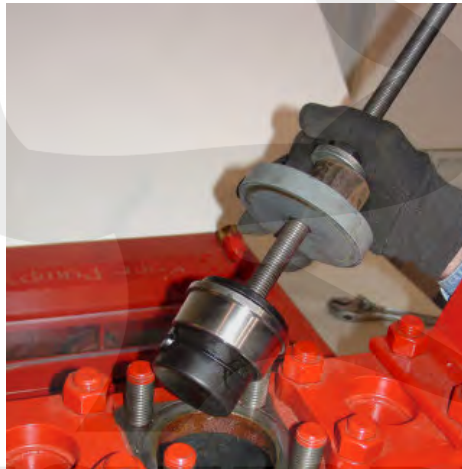
11.) Remove the puller assembly with seat attached.
