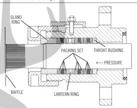
Above depicts Styles 838 and 858 packing correctly installed with all packing lips facing **TOWARD** the fluid pressure. Note that two (2) units of Styles 838 and 858 packing are positioned ahead of the lantern ring, and one (1) unit is positioned behind it. Thus lubricant entering the lantern ring is forced toward the pressure.
