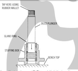
Apply oil liberally to plunger O.D. and lightly tap it through the packing. When introducing the plunger through the MA-155M stuffing boxes, also apply oil liberally to the O.D. of each extension rod to allow easy passage through the wiper box seals.
