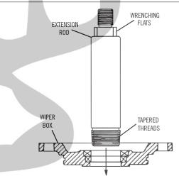
Insert the extension rod through the wiper seals with the tapered thread and entering **FIRST**. Care should be used in moving the extension rod through the seals with wrenching flats entering first. **Do not force!** The sharp corners on the wrenching flats may damage the seal lips! (Resulting in oil leakage.)
