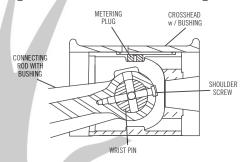
The hole in the wrist pin should line up with the hole in the connecting rod. Install the shoulder bolt through the wrist pin and thread into connecting rod.
