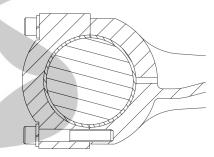
Check that all oil holes are clean and fully open. GRIT is the greatest enemy of bearings, however precisely manufactured. Hence, all surfaces must be perfectly clean and lightly oiled prior to assembly. Remove any burrs or sharp corners which prevent the perfect fitting of these precision bearings. Using a torque wrench, tighten cap bolts as follows:
