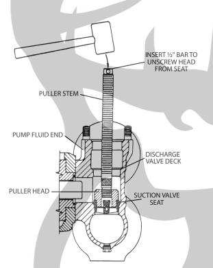
The puller stem and puller head are provided with tapered (locking) threads. Screw them together using two pipe wrenches applied to the knurled areas provided. Then screw the valve seat onto the puller head by hand until it shoulders against the puller shoulder. Do not tighten.
