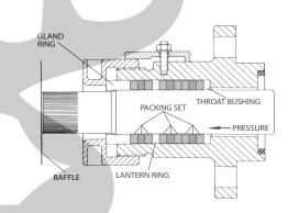
The above depicts Style 838 and 858 packing correctly installed with all packing lips facing *toward* the fluid pressure. Note that two (2) units of Style 838 and 858 packing are positioned ahead of the lantern ring, and one (1) unit is positioned behind it. Thus lubricant entering the lantern ring is forced *toward* the pressure.
