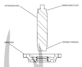
With extension rod inserted through the wiper box seal, thread the tapered threads (must be clean!) into the tapered crosshead female threads. Firmly tighten, apply torque to the wrenching flats only. Never damage the extension rod ground surface!
