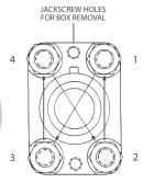
Using a socket, socket extension, and torque wrench, tighten clean, well-oiled threads and nut faces.
