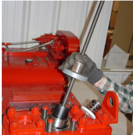
8.) Remove the puller assembly with seat attached.
