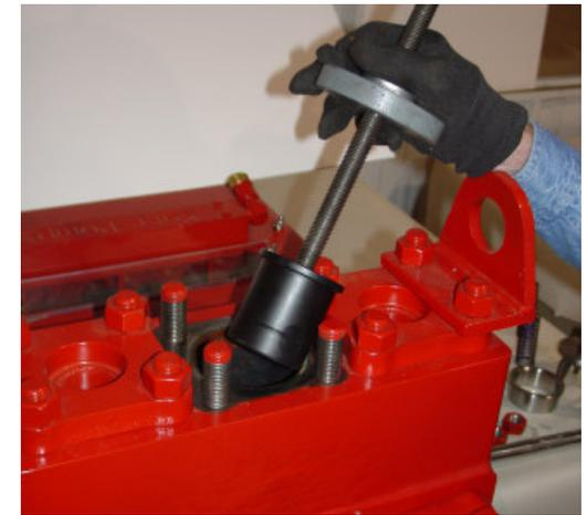
**6.) Insert the tri-pin puller head, all pins retracted, into the discharge seat.**
