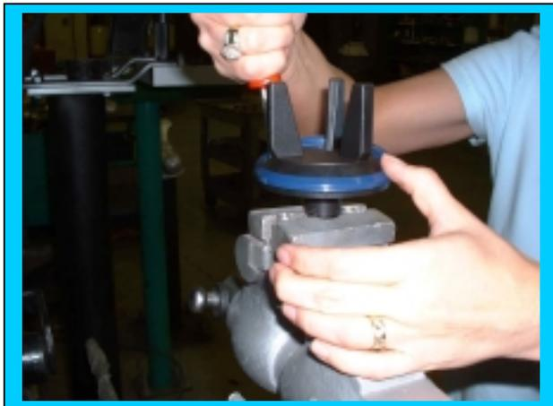
**4) While holding valve down with thumb, rotate around valve with tool. (Similar to mounting a tire on a rim).**
