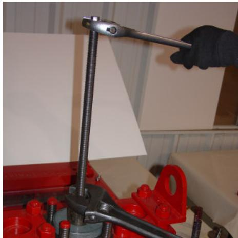
10.) Install seat only in the lower suction location and with an old/used disc on top of the new seat, drive in firmly with a hollow bar.
