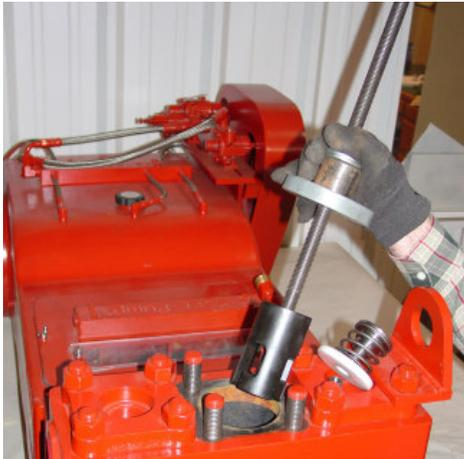
4.) Insert the "J" puller head into and through the discharge seat.
