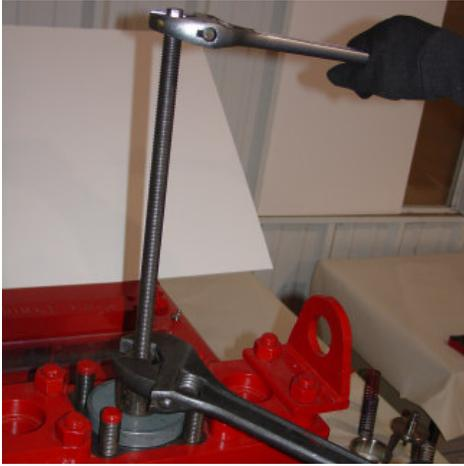
7.) Holding the top of the puller rod in place, tighten the nut until the seat releases.
