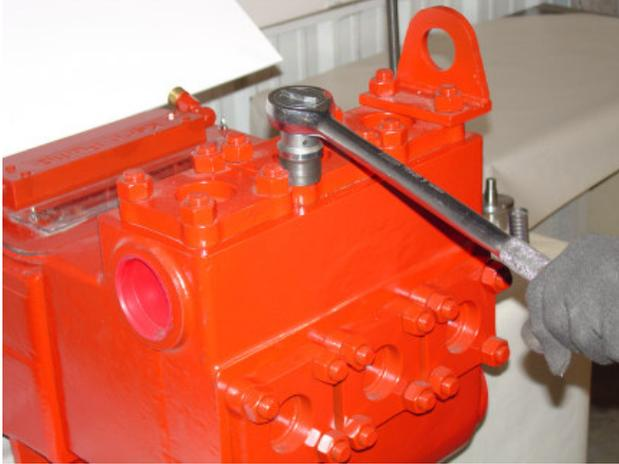
1.) Remove the nuts/cap screws from the top and end covers.
