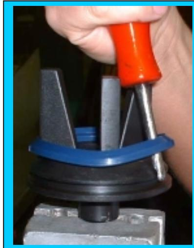
**2) Put Tool between valve and valve insert with groove against valve.**
