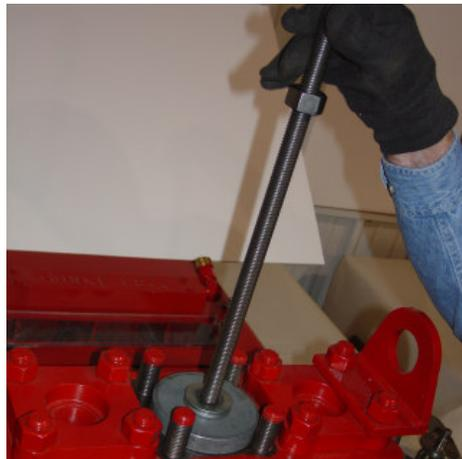
5.) Slide puller plate spacer and washers down the puller rod.
