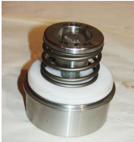
11.) Install the disc sleeve spring, retainer and cap screw. Tighten to the specified torque.
