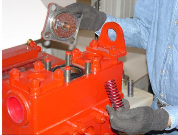
**2.A) Remove the top cover and discharge spring.
