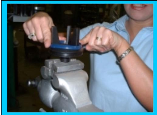
**1) Push Valve Insert over valve legs. Hint: (Insert will be more pliable if heated first-- warm to the touch not hot).**
