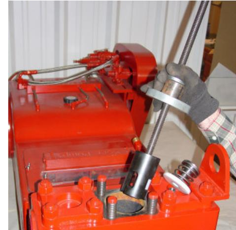
9.) Remove the seat from the puller head and remove the remaining discharge seats
