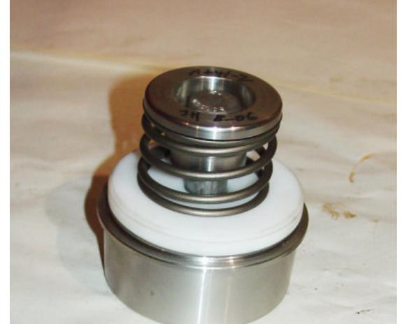
3.) Unthread the discharge valve cap screw and remove with retainer, spring, disc and sleeve.
