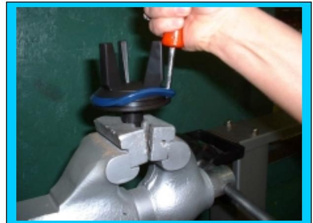
**5) Continue rotating around valve with tool until insert is completely in groove.**
