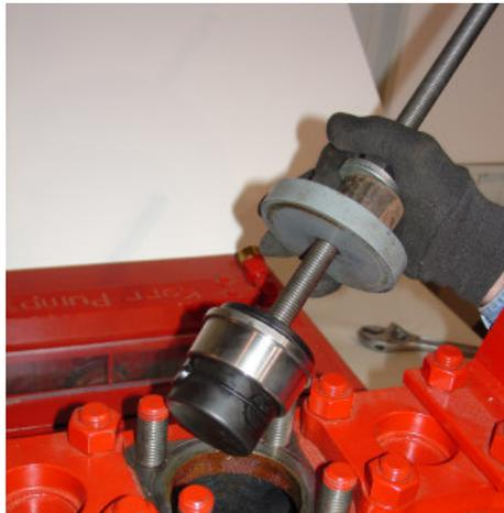
11.) Remove the puller assembly with seat attached.
